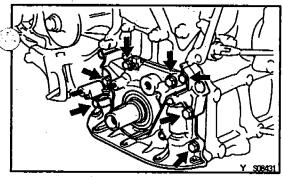
(c) Install the oil pump with the 7 bolts.
